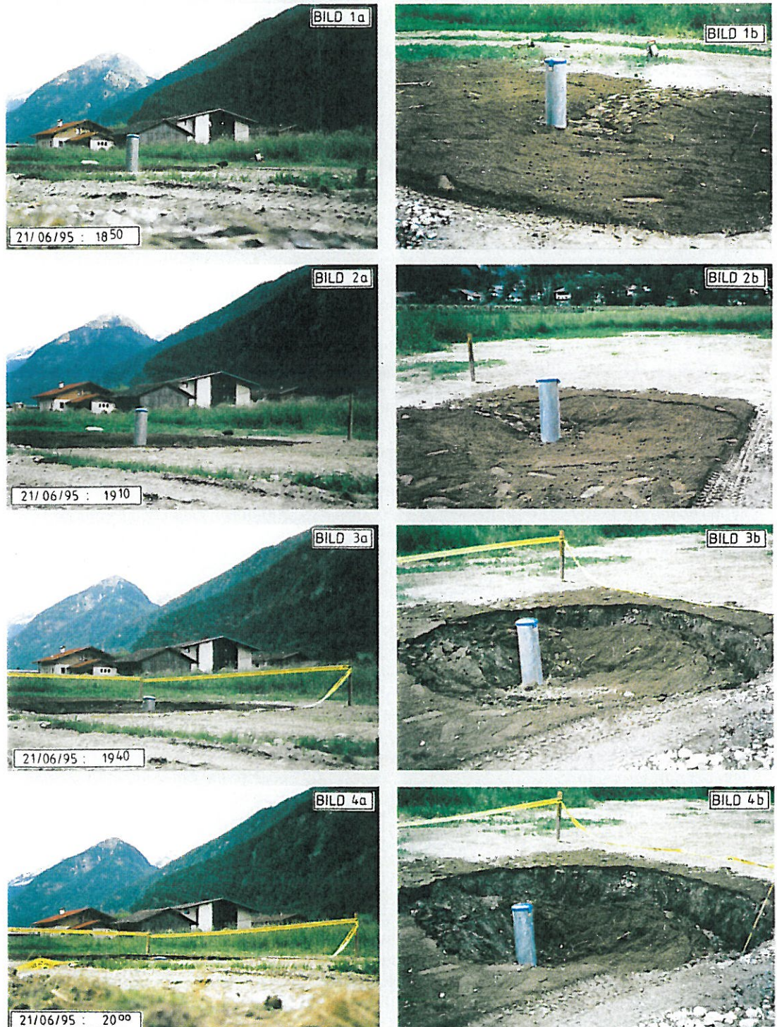
Fig. 1 Initial stages of sink-hole development on June 21, 1995.
